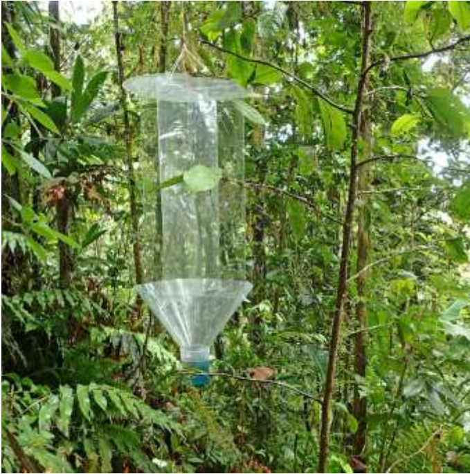
Fig. 3. Piège Polytrap™. Suspended in a favorable location, this trap, composed of transparent plastic plates crossed, intercepts the insects that fly in the environment. These insects hit the vertical plate and then fall into the collection pot filled with a preservation liquid.
