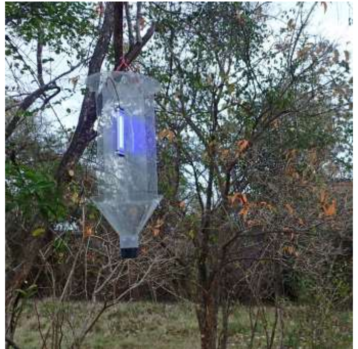
Fig. 4. Piège Polyvie bleu (PVB). This trap is the subject of developments by SEAG since 2010. It combines the interception effect of a Polytrap™ trap and a luminous attraction of low power that works on battery with a programmer. The blue LED ramps (aquariophilia) offer a particular luminous spectrum that has proved effective in Guyana and the Antilles.
